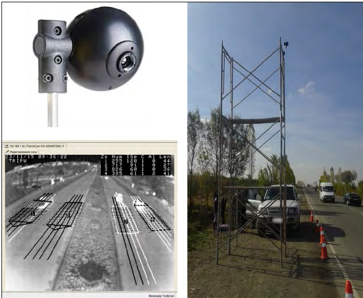
Figure 5.2-1 24-Hour Screenline Survey Using a Thermal Camera
