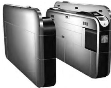
Fig. 6-7-18 AFC equipment as advanced electronic equipment (example of an automatic ticket gate)
