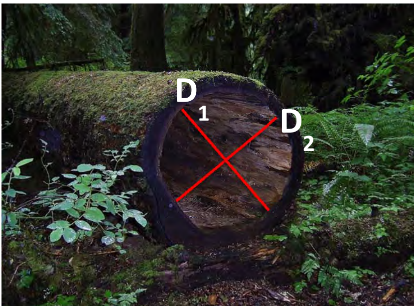
Figure 15 Hollow Log. Two measurements of the diameter of the hollow shall be taken
