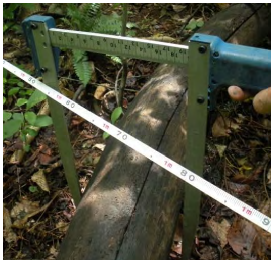
Figure 13: Use of calipers to measure the diameter of lying deadwood along line transect
