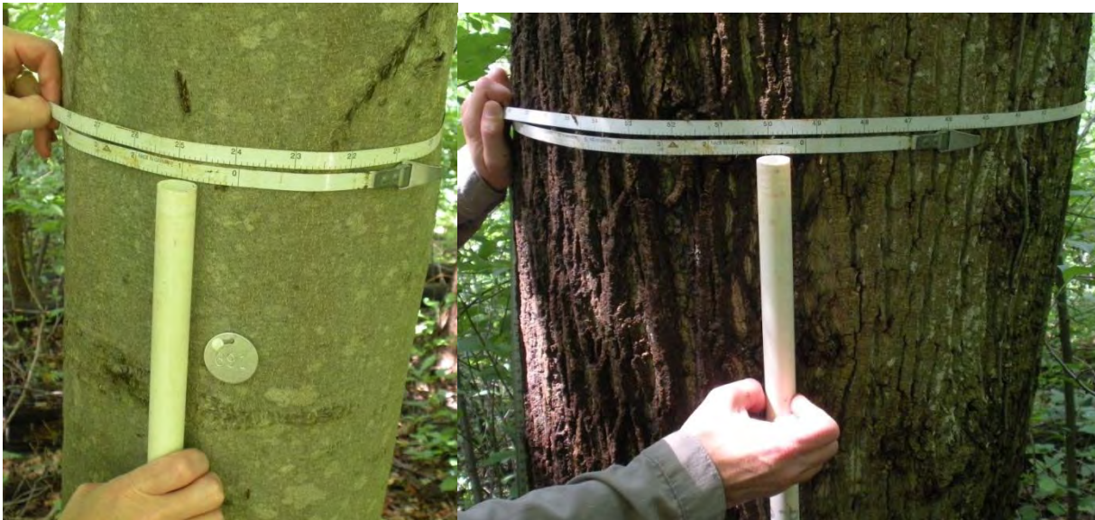
Figure 12: Measurement of diameter using a diameter tape and tree pole
