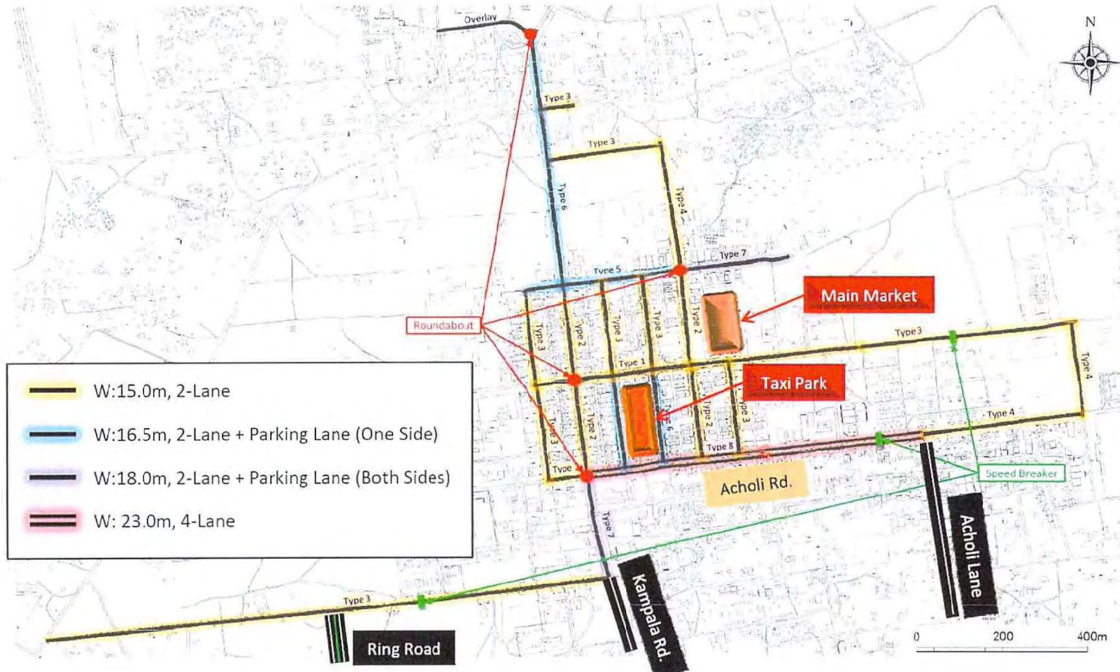
Figure 3.2 Typical Sections of Target Roads
