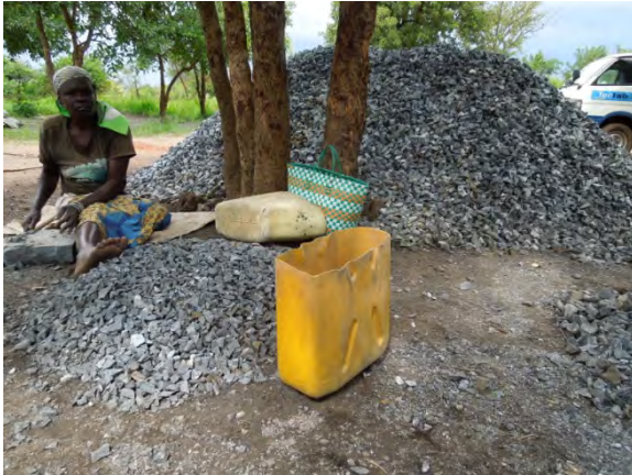
Conditions for manual production of crushed rock
