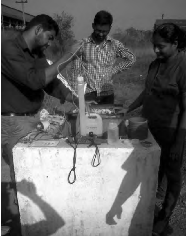
Picture 3.1. Test Well Water Collection using Bailer
