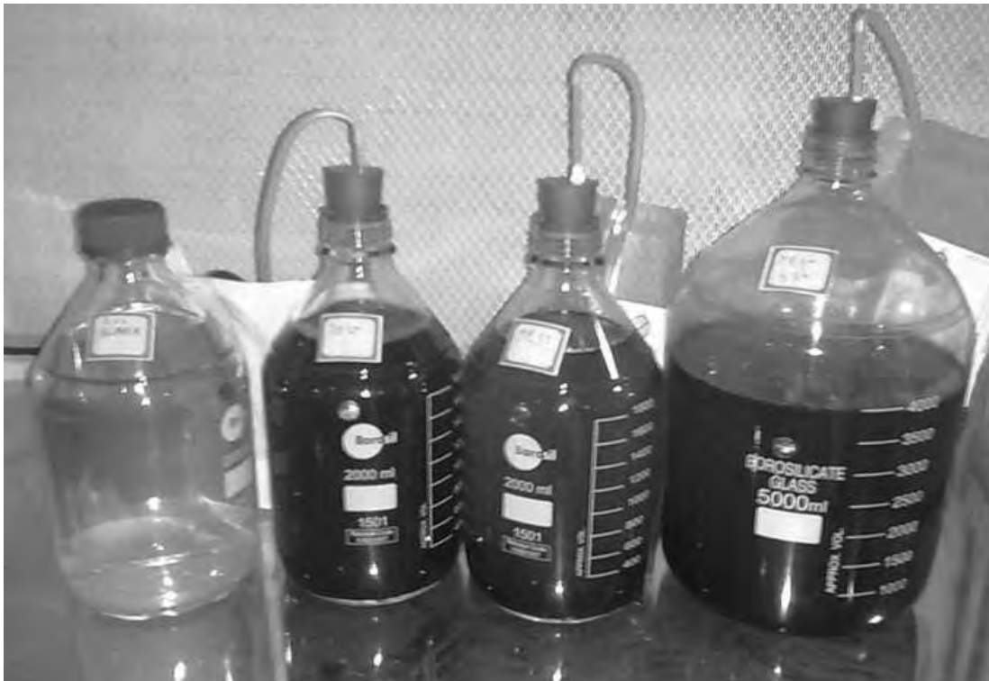
Picture 3.6. Comparison microcosm test one month after nutrients and pH buffer added to hexavalent chromium contaminated water with control (yellow color water on the left side of the picture)
