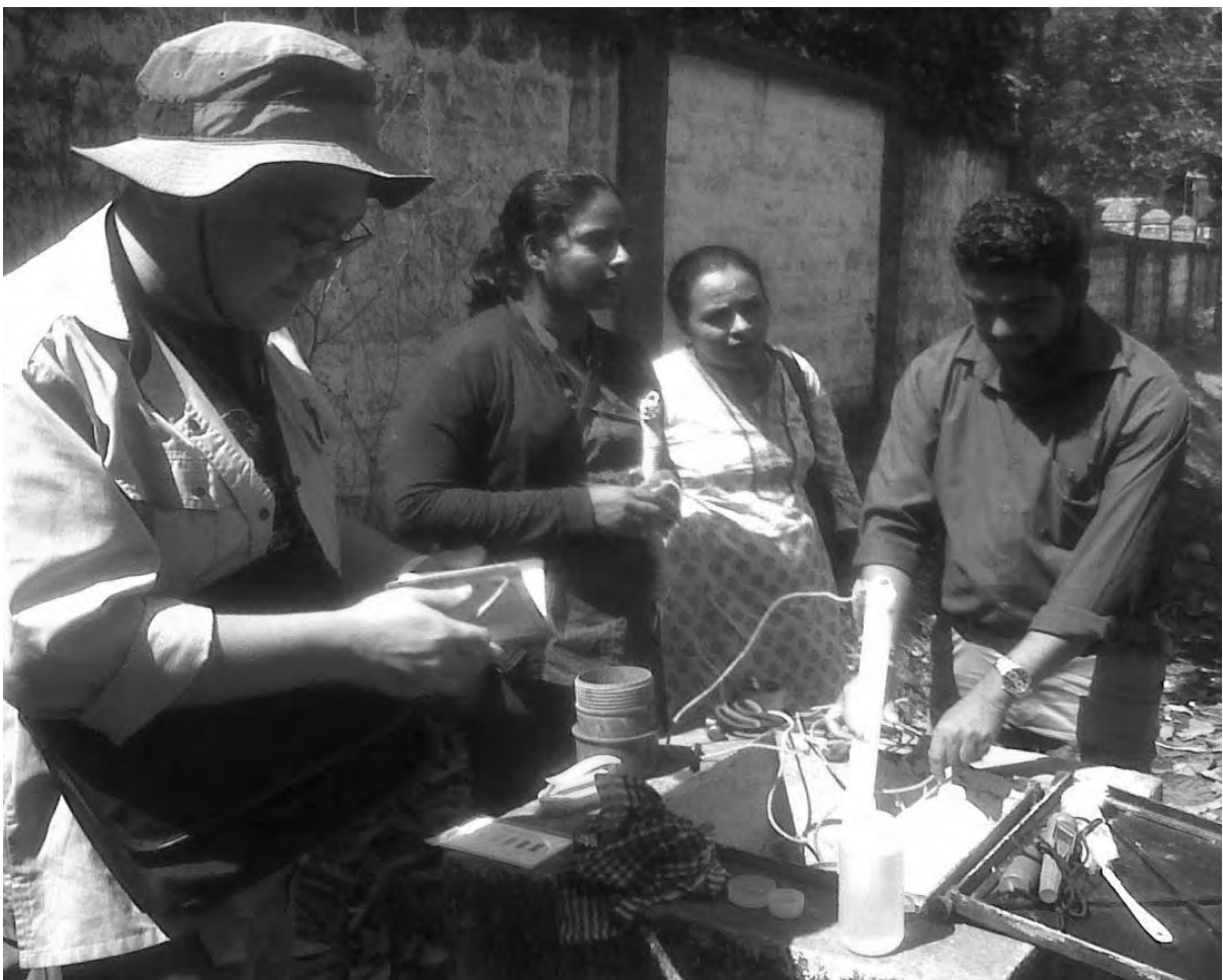
Picture 1.1. Groundwater Sampling by Bailer Using Test Well in Cuncolim Industrial Estate.
