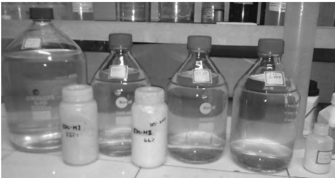
Picture 3.4. Bethora Industrial Estate Groundwater Mixed with Aero Coach Electroplating Effluents and with Hexavalent Chromium Before EDC-M1 & EDC-M2 Nutrients Addition
