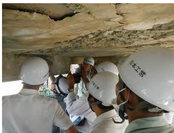
Photo 3.20 Demonstration of Rebar Detection and the Trainees' Operation of the Equipment
