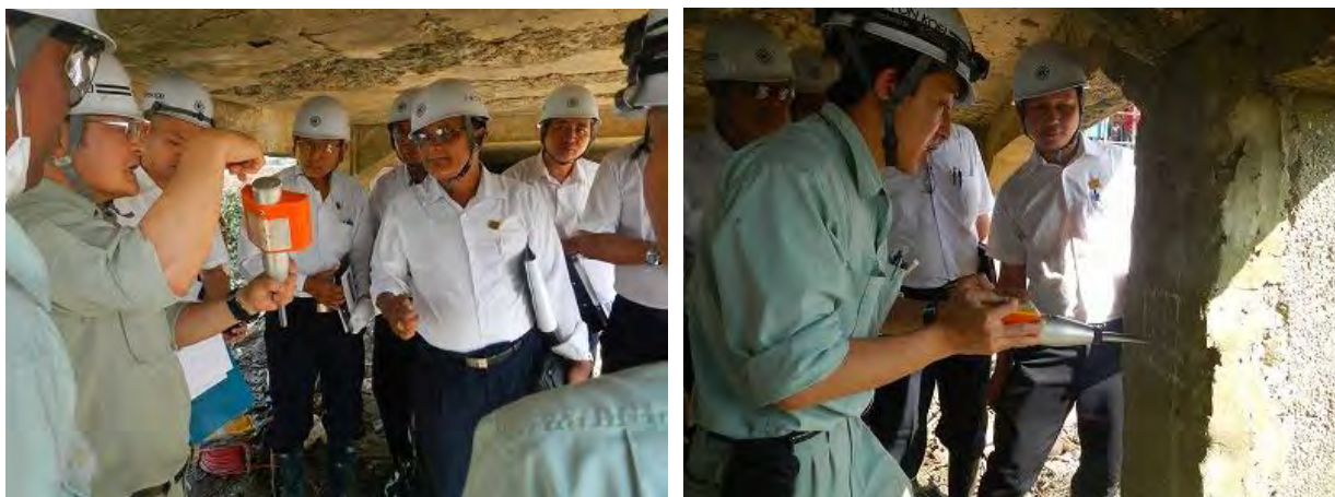
Photo 3.17 Explanation and Demonstration of the Schmidt Hammer Test
