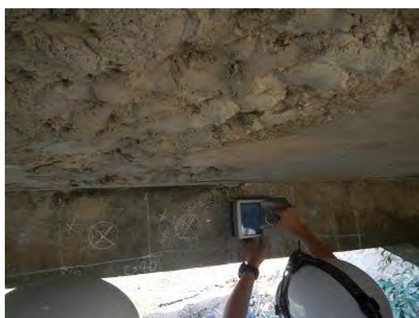
Photo 3.20 Demonstration of Rebar Detection and the Trainees' Operation of the Equipment
