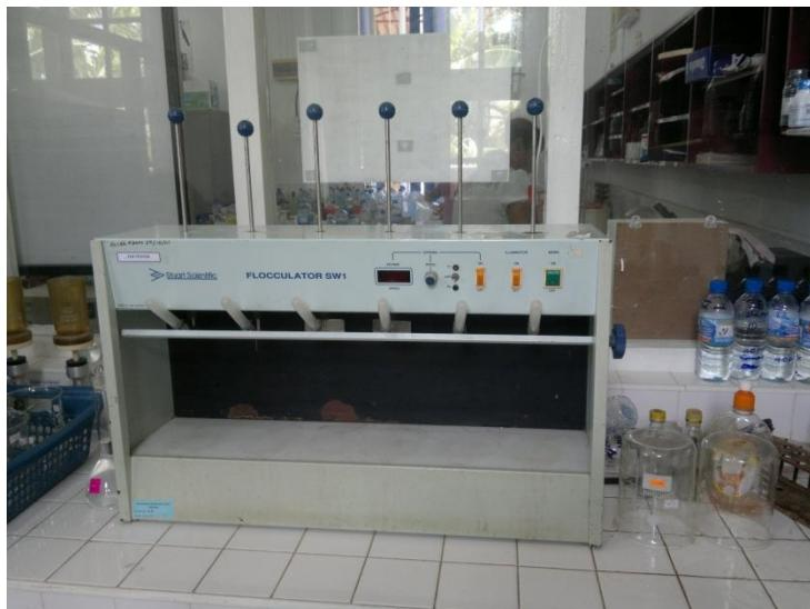
**Equipment Used for Jar Testing**
