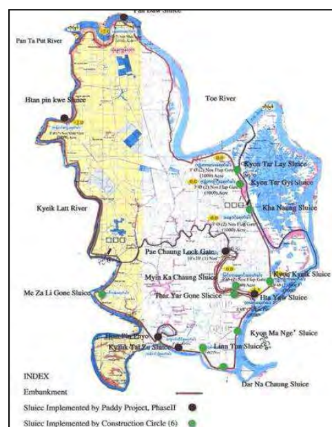
Figure 3.3.34 Tonegwa Polder Irrigation System
