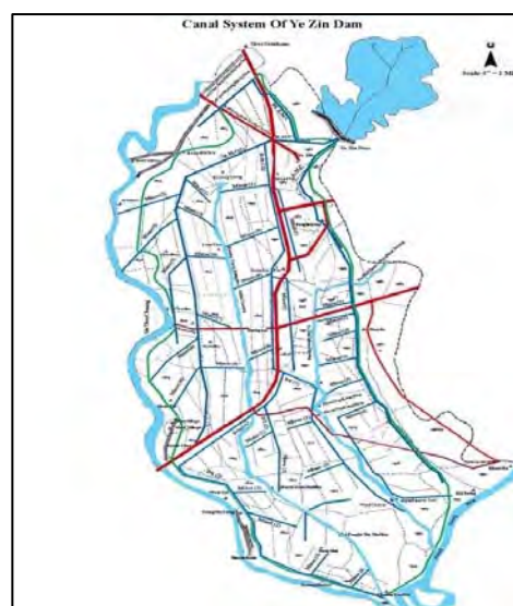
Figure 3.3.12 Yezin Dam Irrigation System
