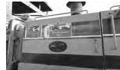
Safety Posters Placed on Machines should be standardized and placed in same locations
