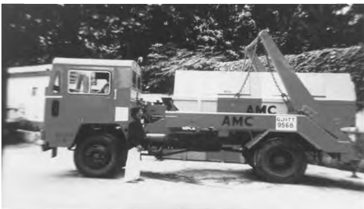
Dumper placer container ready for transportation
