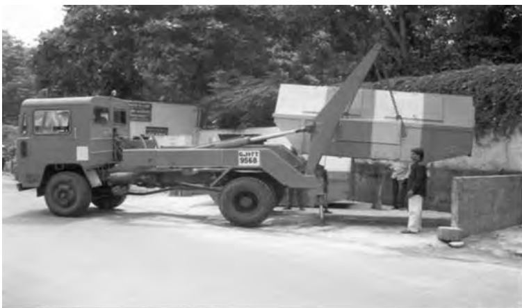
Dumper placer bin lifting system
