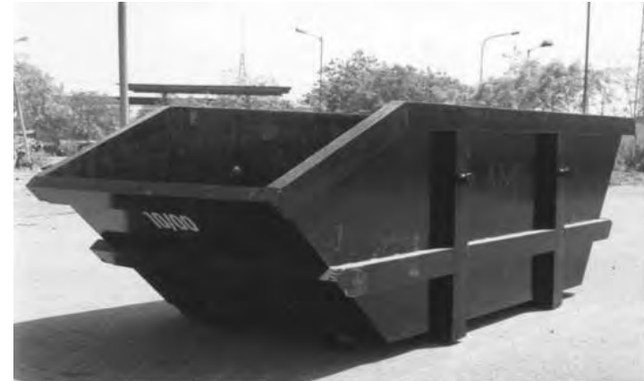
Skip (container) meant for the storage of construction/demolition waste.
