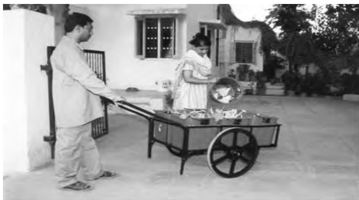
Use of containerized handcart/tricycles for door to door collection of waste
