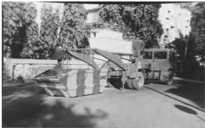
Lifting of skips through contracting mechanism
