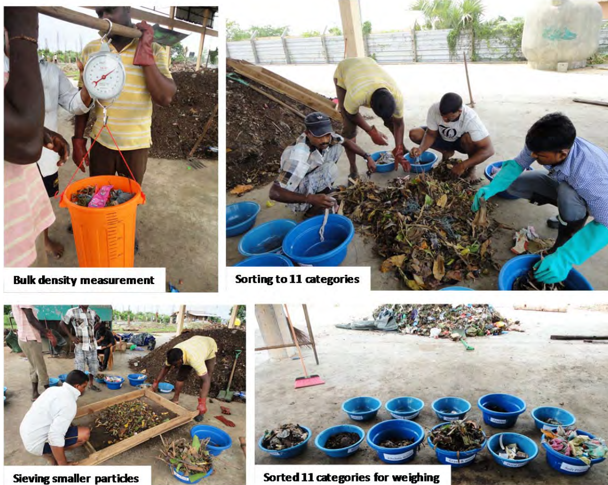
Figure 2-3 Procedure of analysis of physical composition
