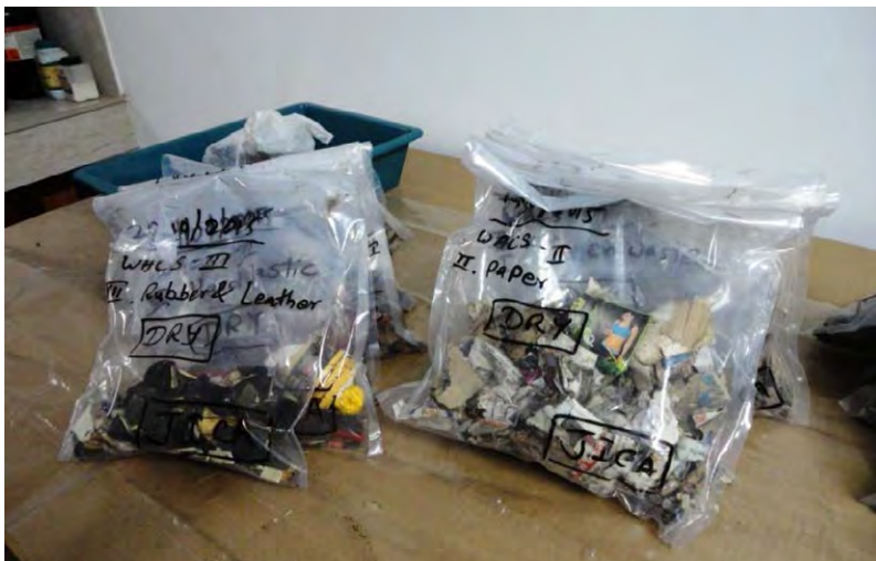
Figure 2-4 Dried waste samples at laboratory is ready for sealed packing after water content analysis
