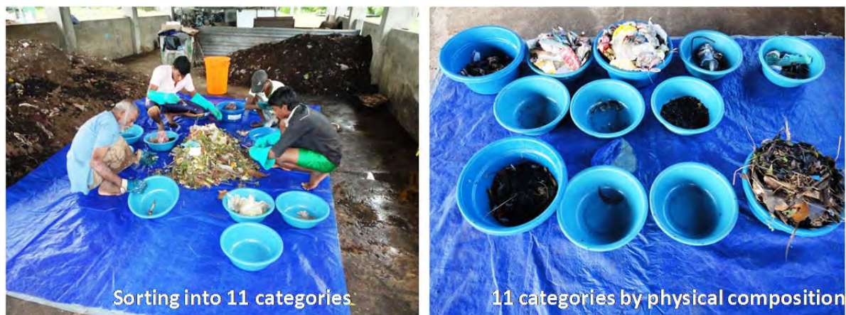
Figure 2-3 Procedure of analysis of physical composition
