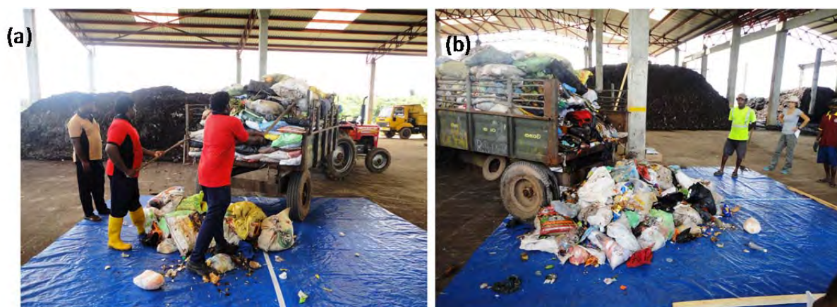
Figure 2-1 Sampling for WCS at DMMC, (a) manually unloading the profile sample and (b) unloaded sample
