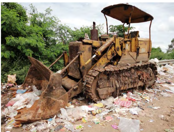
Figure 4-5 Bulldozer is employed for waste handling at KSUC dumpsite
