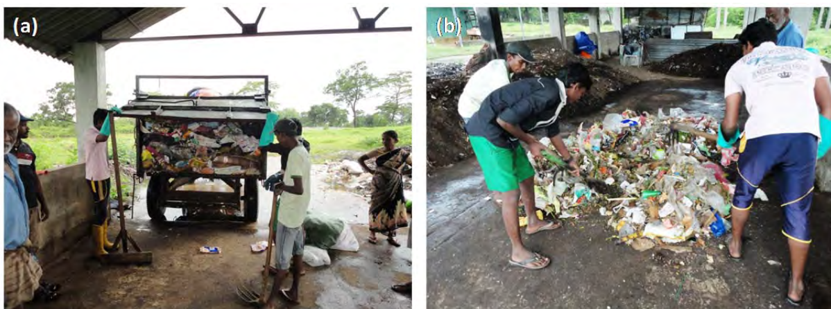
Figure 2-1 Sampling for WCS at TPS, (a) manually unloading the profile sample and (b) unloaded sample
