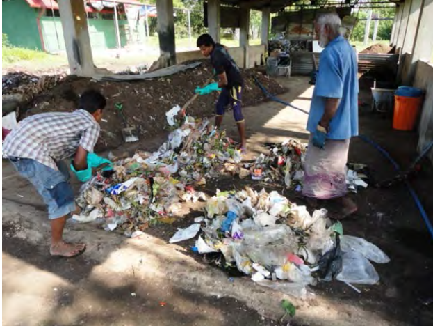
Figure 2-2 Particle size reduction, mixing and preparation of working sample by coning & quartering technique
