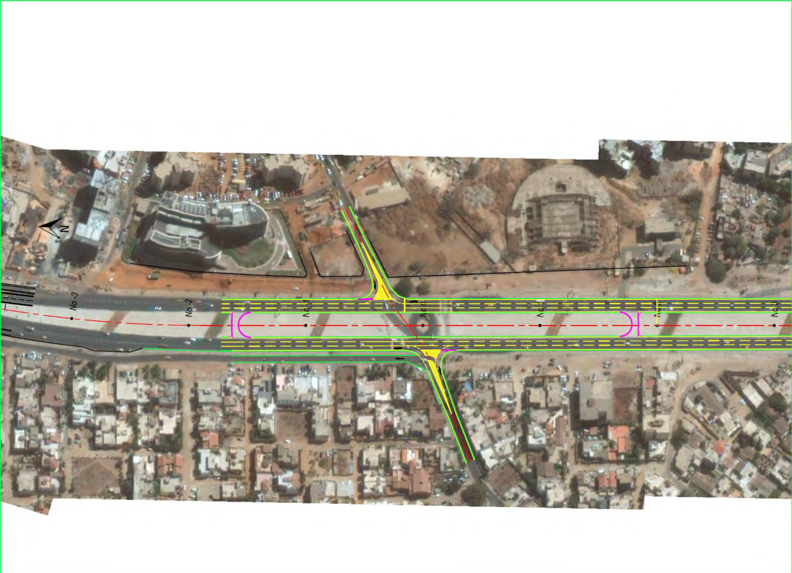
Figure 12.5.12 At-grade Improvement with U-turn Lanes at Cité Keur Gorgui (I-02f)
