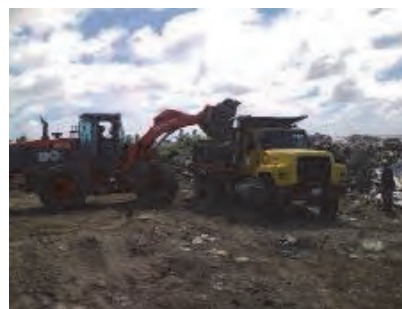
Scattered waste was loaded to the dump truck by the wheel loader
