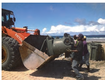
Waste collection method using a wheel loader and a dump truck
