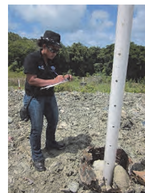
Monitoring gas temperature
