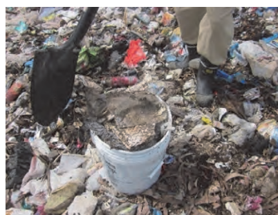
Measuring compaction ratio at dumpsite
