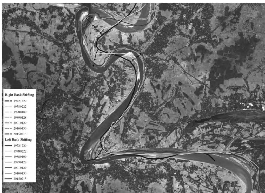
Figure 5.4.29 Shifting of Left Bank Lines around the Kalna Bridges during Past 43 years
