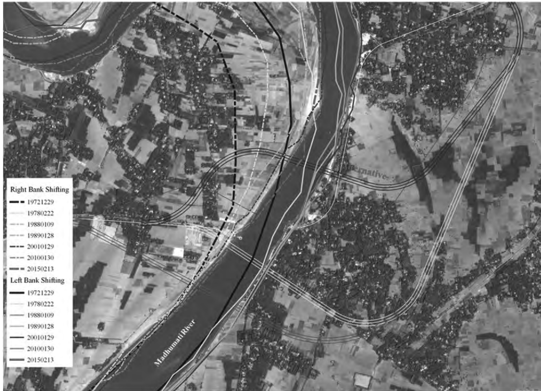
Figure 5.4.27 Zoomed View of Shifting of Bank Lines around the Kalna Bridges during Past 43 years
