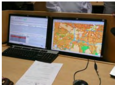
Figure 20. Controller Graphic interface showing in-service bus log and real-time location map
