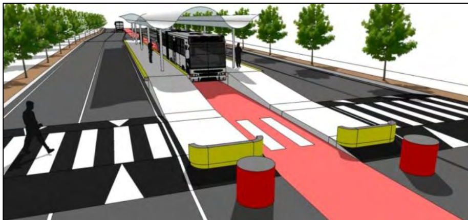
Figure 11. Station showing raised pedestrian crossing and access ramps
