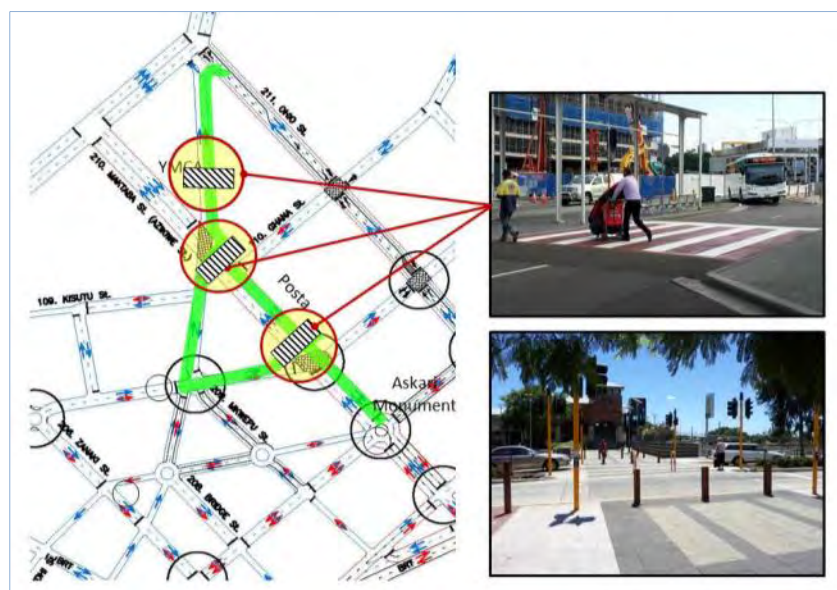
Figure 7.2.5 showing location & design of raised crossings
