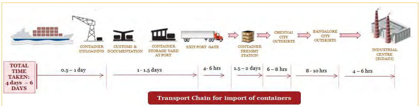
Figure 6.7.4: Chain of activities taking place in import and export of containers
