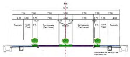
Figure 7.17: Proposed Typical Cross Section (Primary-4 Lanes)
