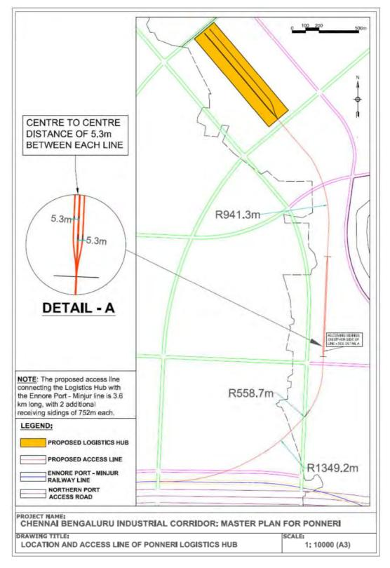
Figure 7.35: Ponneri Node – Layout of proposed rail access line and reception sidings
