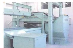
Magnetic separator -Sorting by magnetic forces
