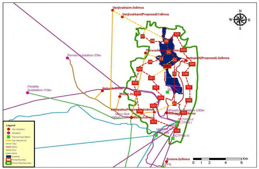
Figure 7.43: Sub-station locations for Phase III
