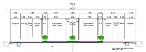
Figure 7.20: Proposed Typical Cross Section (Primary-Residential-4 Lanes)
