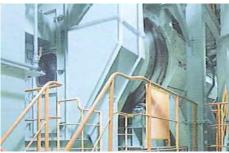
Trommel screen -Sorting by the particle size and wind
