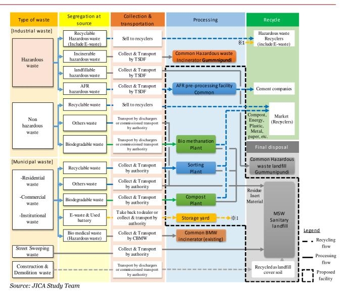
Figure 1.14: Solid waste management in the Nodefor the Phase 3
