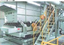
Vibration & wind separator -Sorting by vibration and wind
