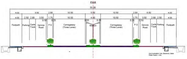
Figure 7.18: Proposed Typical Cross Section (Primary-Residential-6 Lanes)
