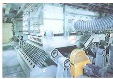
Jumping screen -Removing the moisture and dust by jumping
