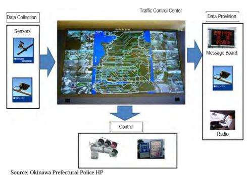
Figure 7.11: Integrated Traffic Control System
