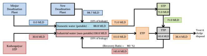
WTP: Water Treatment Plant, STP: Sewage Treatment Plant, ETP: Effluent Treatment Plant, TTP: Tertiary Treatment Plant for Recycling of sewage and industrial wastewater
