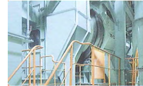
Trommel screen -Sorting by the particle size and wind
