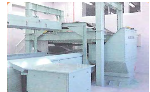
Magnetic separator -Sorting by magnetic forces
