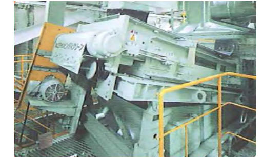
Incombustible separation machine -Sorting by crushed and reclaimed sand
