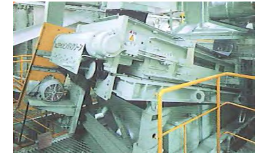
Incombustible separation machine -Sorting by crushed and reclaimed sand
