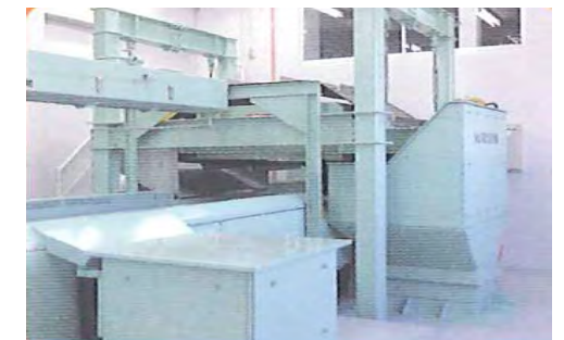
Magnetic separator -Sorting by magnetic forces
