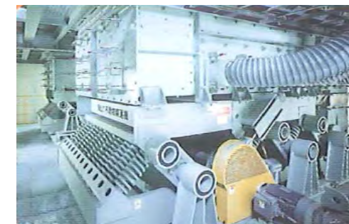
Jumping screen -Removing the moisture and dust by jumping
