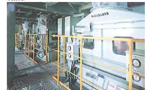
Specific gravity separator - Sorting by the weight difference
