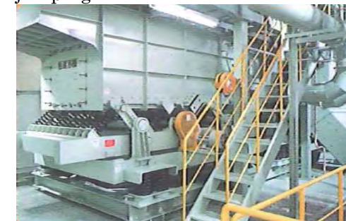
Vibration & wind separator -Sorting by vibration and wind
