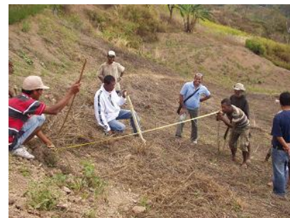
A one-meter stick should be used to check the vertical distance between contour lines.
