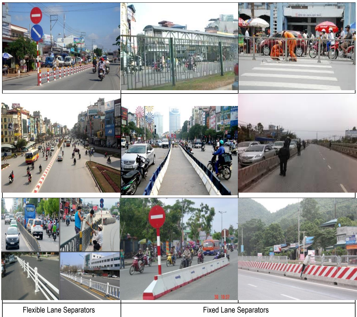
Figure 2.2.26 Various Types of Lane Separators
