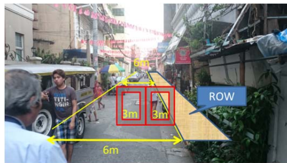
Figure 3.2.10 ROW and Resettlement
