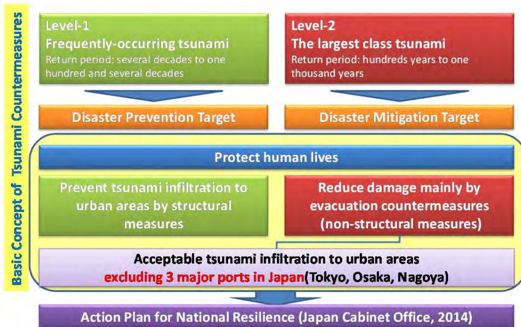
Figure 6.1-12 Clarification of Disaster Prevention Level against Tsunami
