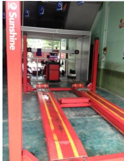
Alignment measuring facility
