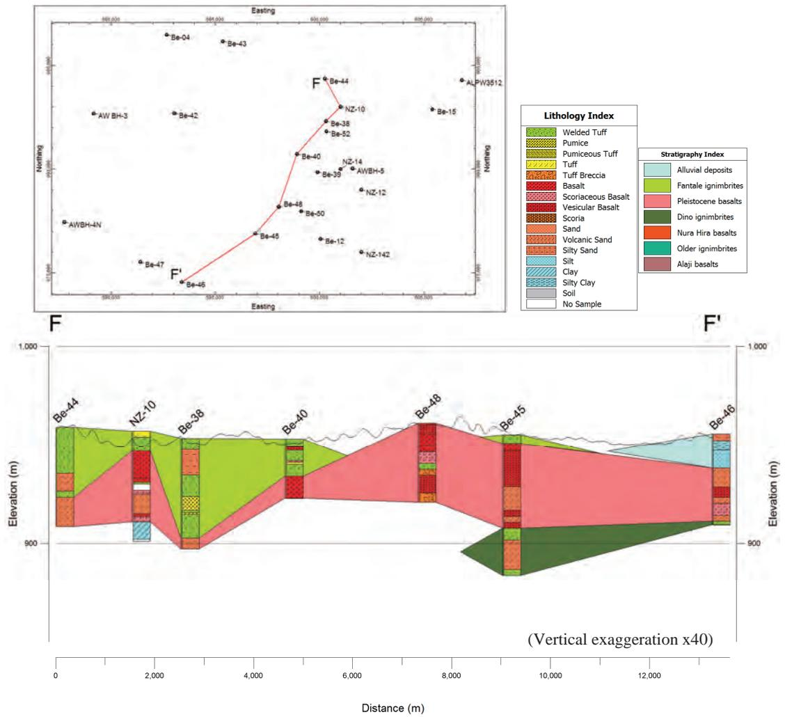
Figure 5.1.28: Borehole log profile F-F' section
