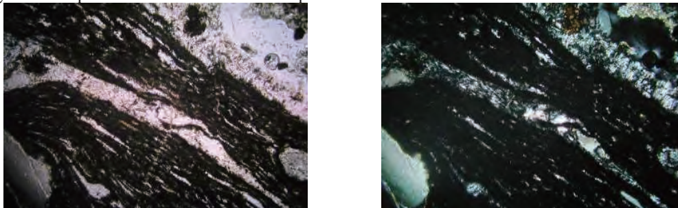
Base of photo 0.8mm: Welded glass shards and flattened pumice. Crystallization of zeolite as fibrous aggregates from the edges towards the centers of lenses could be caused by diagenesis. This rock is considered to be a member of older complex.
