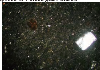
Base of photo 0.7mm: Matrix of welded glass shards and fragments of alkali feldspar and rhyolite. Grasses are dark in crossed polars indicates optical isotropism.
