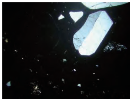
Base of photo 1.6mm: Coarse-grained euhedral alkali feldspars are characteristic. Lens of obsidian is upper left to the center of the photo. Glass shards are welded.
