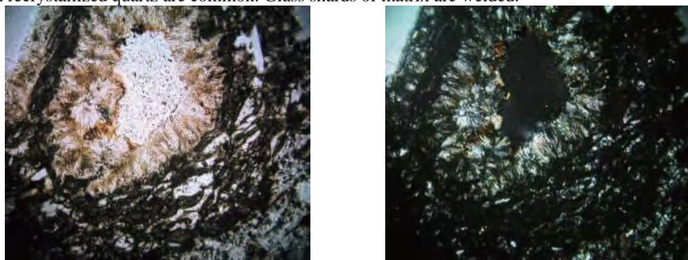
Base of photo 0.7mm: Zeolite occupied a rounded pore. Very fine-grained quartz is formed in welded glass shards. These mineralization is considered to be formed under diagenesis caused by a heat and vapor in the hot pyroclastic flow unit.
