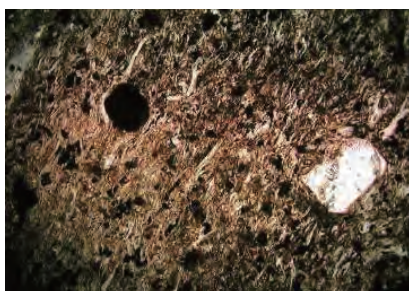
Base of photo 0.7mm: Matrix of welded glass shards and fragments of alkali feldspar and rhyolite. Grasses are dark in crossed polars indicates optical isotropism.
