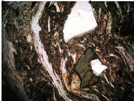
Base of photo 0.8mm. Fragments of alkali feldspar and amphibole. Welded glass shards of matrix are dark in crossed polars which indicates little effect of diagenesis.
