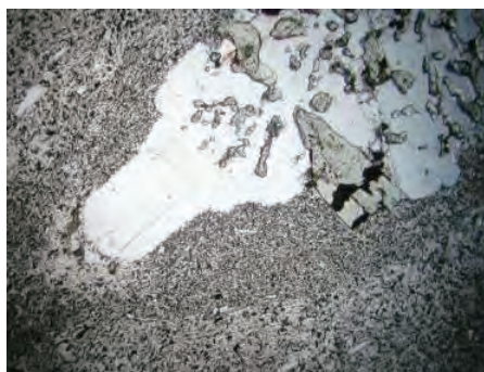
Base of photo 1.5mm: Phenocryst of alkali feldspar including pyroxenes. In groundmass, flow structure is defined by layer of different size of crystal.
