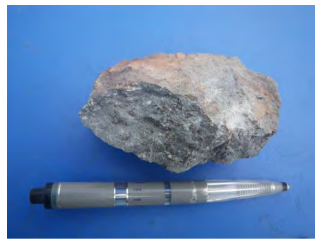
The unit consists of dark gray, porphyritic trachytes. Mt. Zikwala (L-MAD41)
