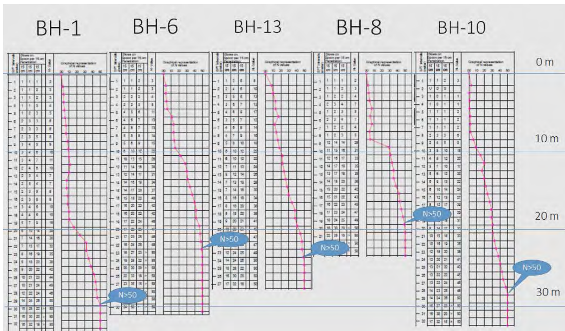
Figure 8.3-4 Representative SPT profiles along the T/L route
