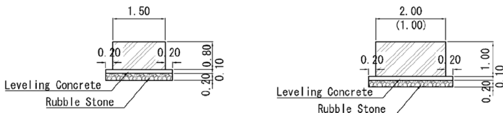
Concrete Foundation for RTG Passing Line
