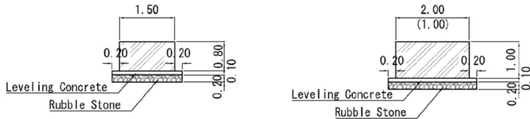
Concrete Foundation for RTG Passing Line
