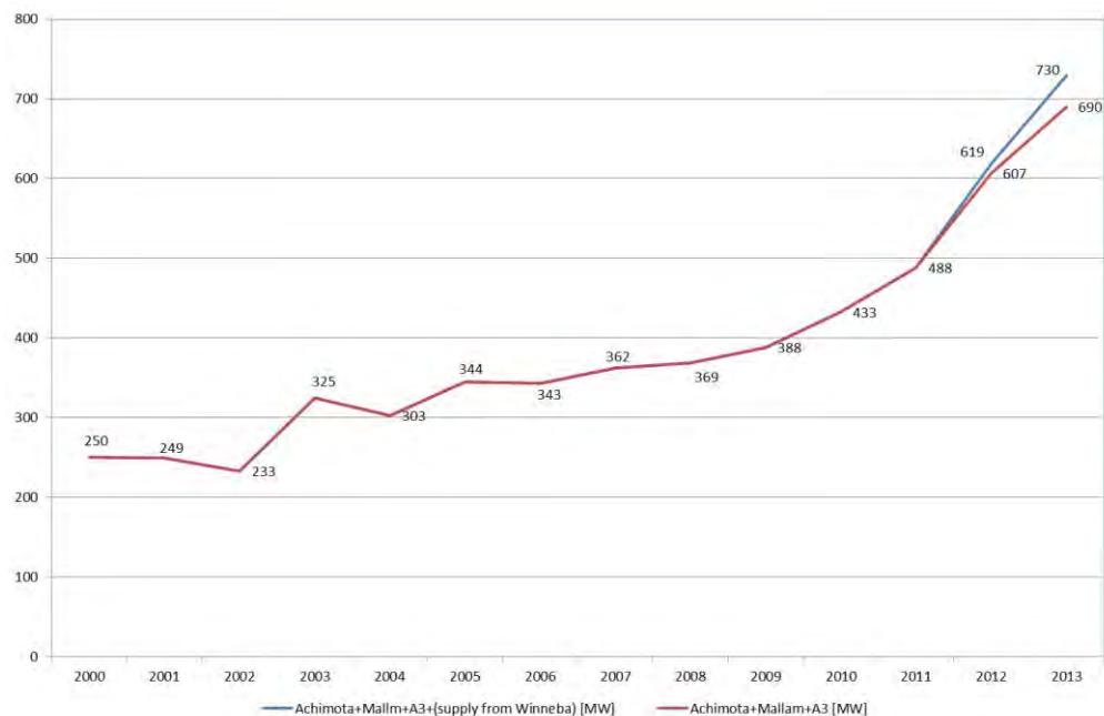
Figure 2-2-2-1.2 Change of Total value of the yearly peak loads of 161 kV Bus in Accra area
