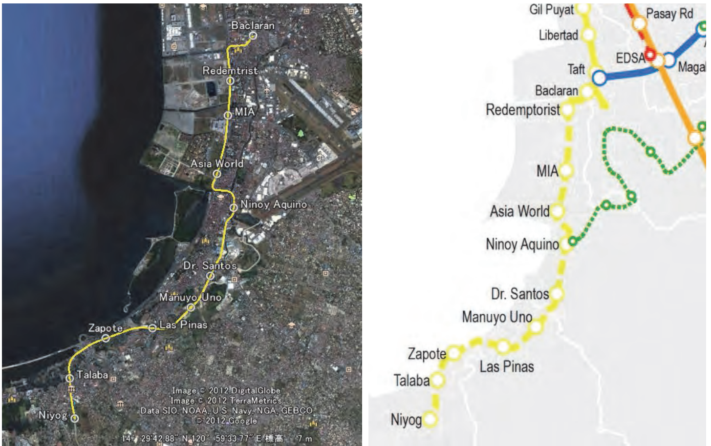
Figure 2.20: Line 1 South (Cavite) Extension Project Proposed Alignment
