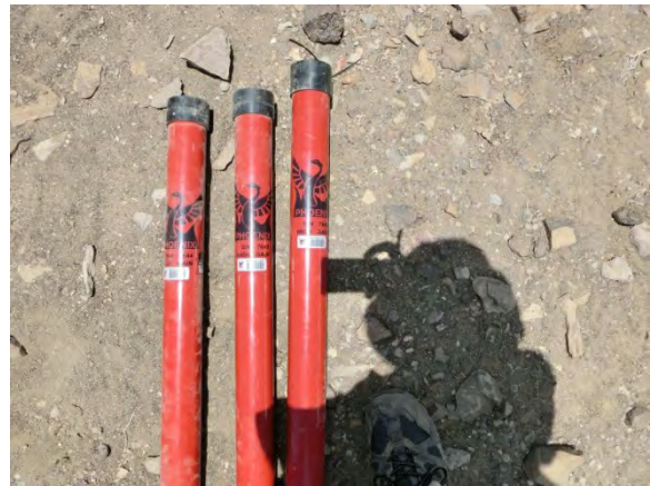
MT/TEM survey: induction coils by Phoenix
