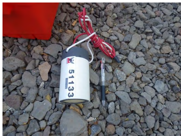
MT/TEM survey: non-polarized electrode
