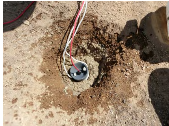
MT/TEM survey: setting of non-polarized electrode
