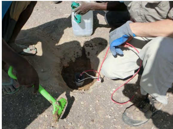
MT/TEM survey: preparation for setting of non-polarized electrode
