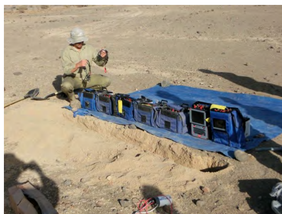
MT/TEM survey: preparation of survey equipment at the site (batteries and data loggers)
