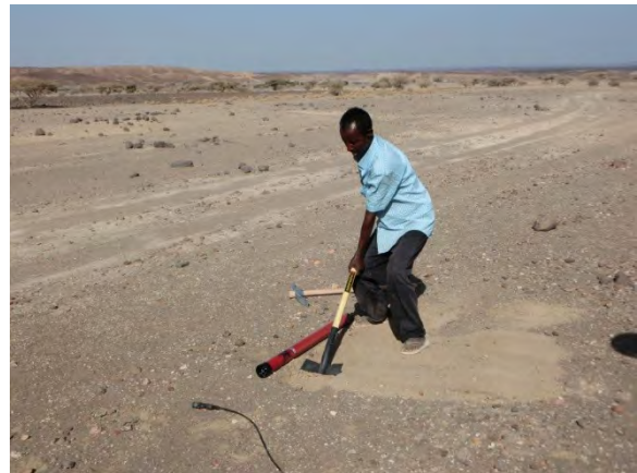
MT/TEM survey: setting of horizontal induction coil
