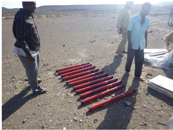
MT/TEM Survey: preparation of induction coils
