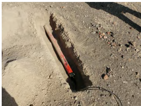
MT/TEM survey: setting of horizontal induction coil
