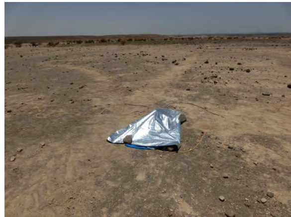
MT/TEM survey: site measurement (data logger was covered by vinyl seat)
