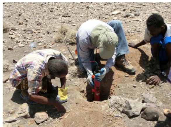
MT/TEM survey: setting of vertical induction coils
