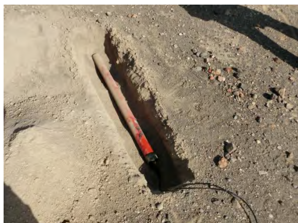
MT/TEM survey: setting of horizontal induction coil
