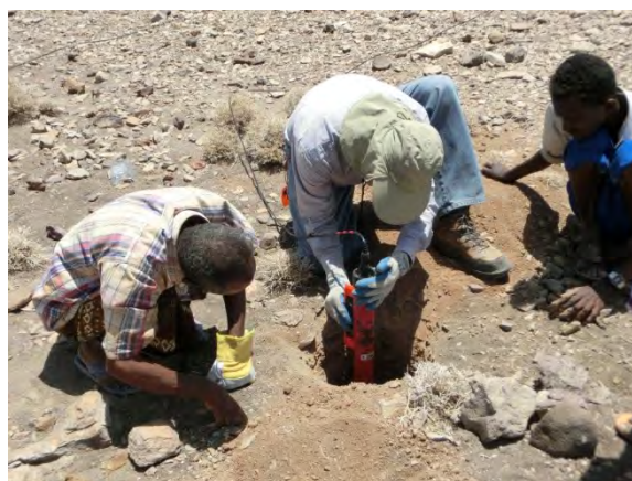
MT/TEM survey: setting of vertical induction coils
