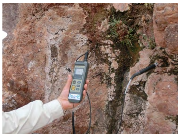
Ground temperature measurement at Garabbayis fumaroles
