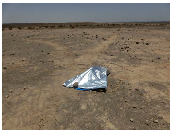
MT/TEM survey: site measurement (data logger was covered by vinyl seat)
