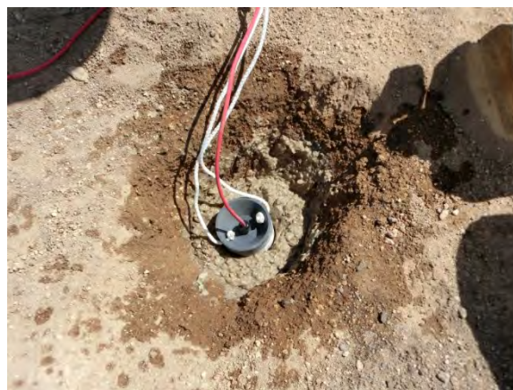
MT/TEM survey: setting of non-polarized electrode
