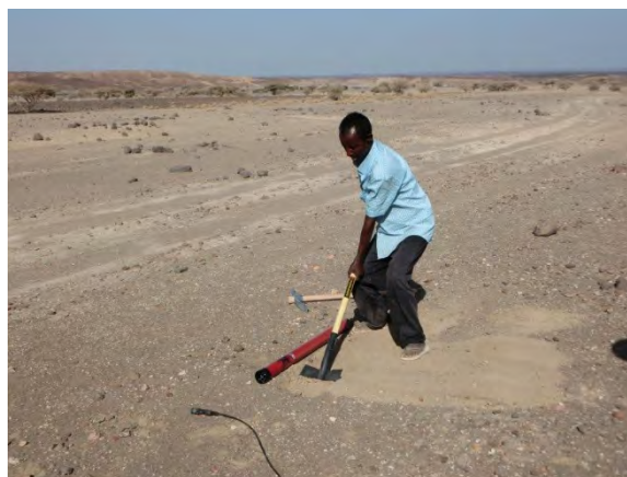
MT/TEM survey: setting of horizontal induction coil
