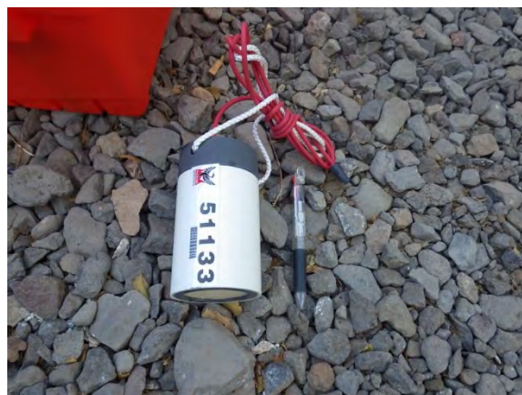
MT/TEM survey: non-polarized electrode
