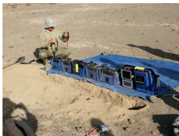
MT/TEM survey: preparation of survey equipment at the site (batteries and data loggers)
