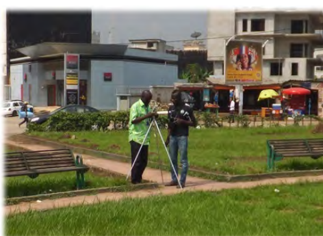
Photo 18 Accuracy Verification of GPS Device Installation (left) and Accuracy Verification of Eccentricity Measurement (right)
