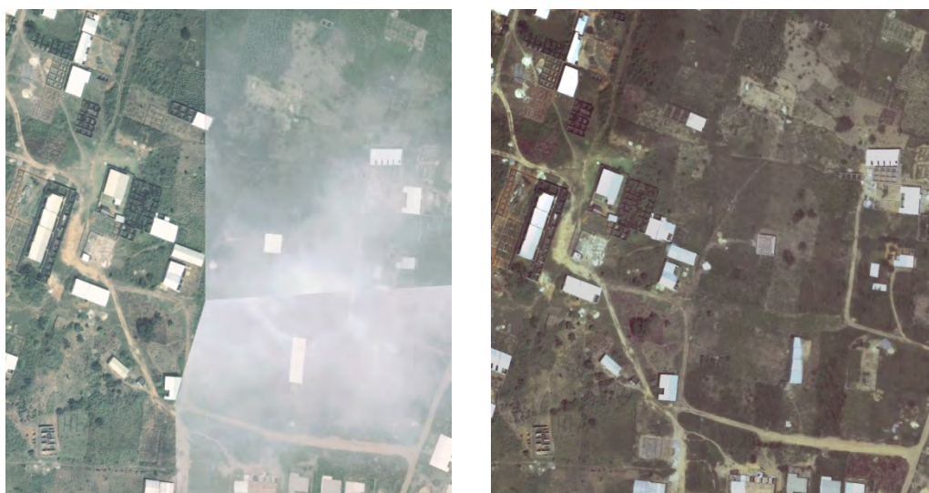
Figure 44 Orthophoto data before correction (left) and Orthophoto data after correction (right)
