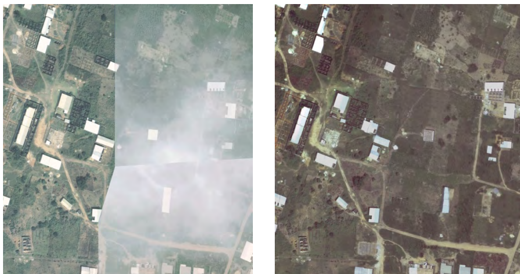
Figure29 Orthophoto data before correction (left) and Orthophoto data after correction (right)
