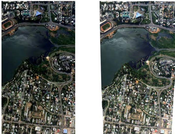
Figure 28 Original Image (left) and Orthophoto Data (right)
