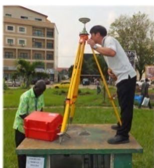
Photo 9 Accuracy Verification of GPS Device Installation (left) and Accuracy Verification of Eccentricity Measurement (right)
