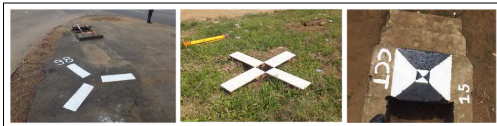
Photo 6 Three Types of Aerial Signal Markings (Types A, B and C)
