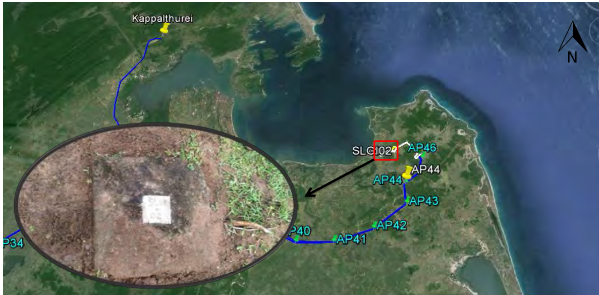
Figure A3 - 1: Control Point “SLGI02” Established by Surveying Department
