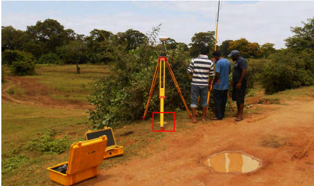
Figure A4 - 5: Establishment of Control Point “LHI02”
