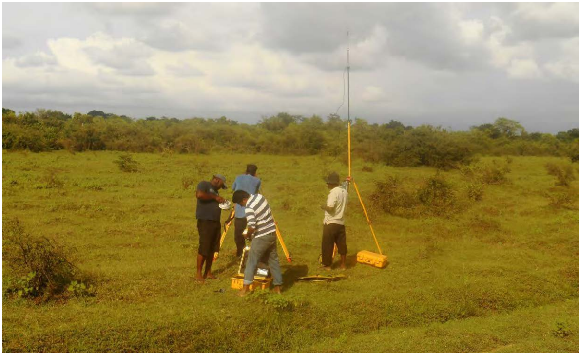
Figure A4 - 2: Establishment of Control Point “LHI01”
