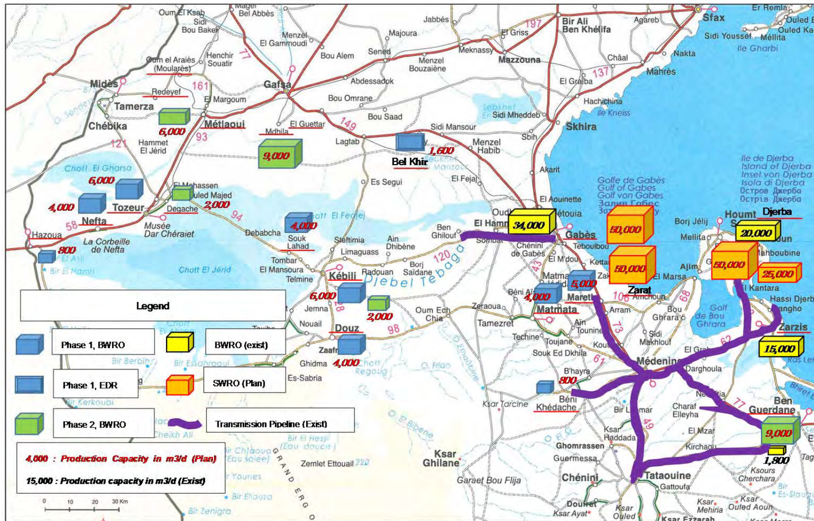
Figure 3.3-25 Desalination plants and water transmission pipelines
