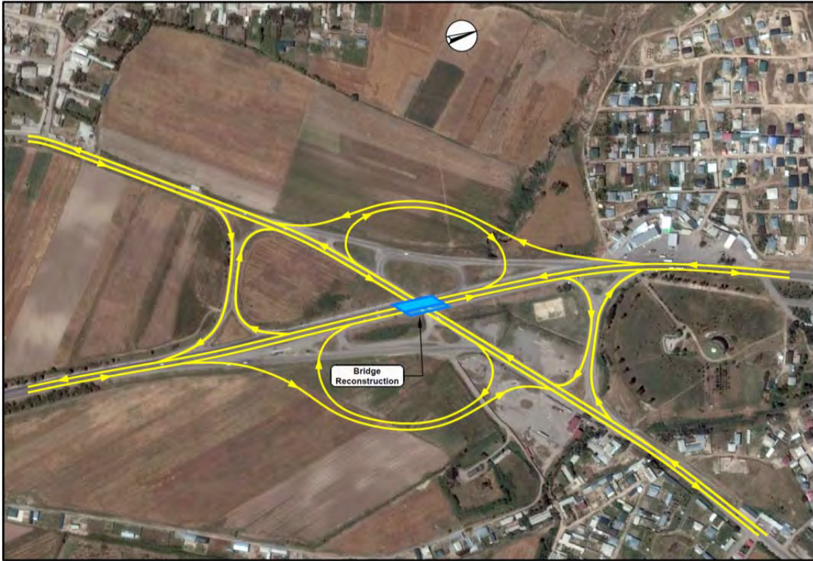
FIGURE 6.12-2 PROPOSED IMPROVEMENT OF INTERCHANGE (KM. 21 + 065)
