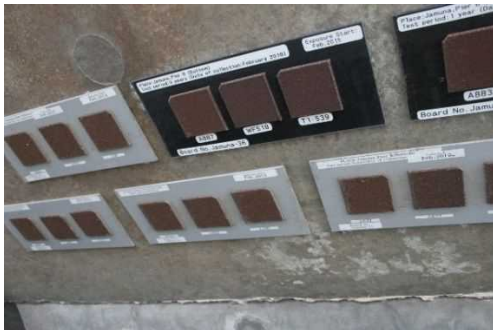
27. Japanese weathering steel plates under exposure test
