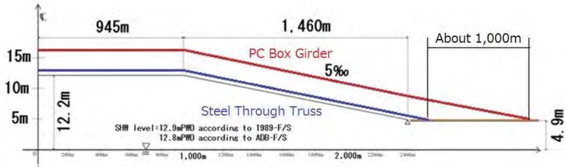
[Fig. 3.4.7] Rail Level Difference according to bridge types
