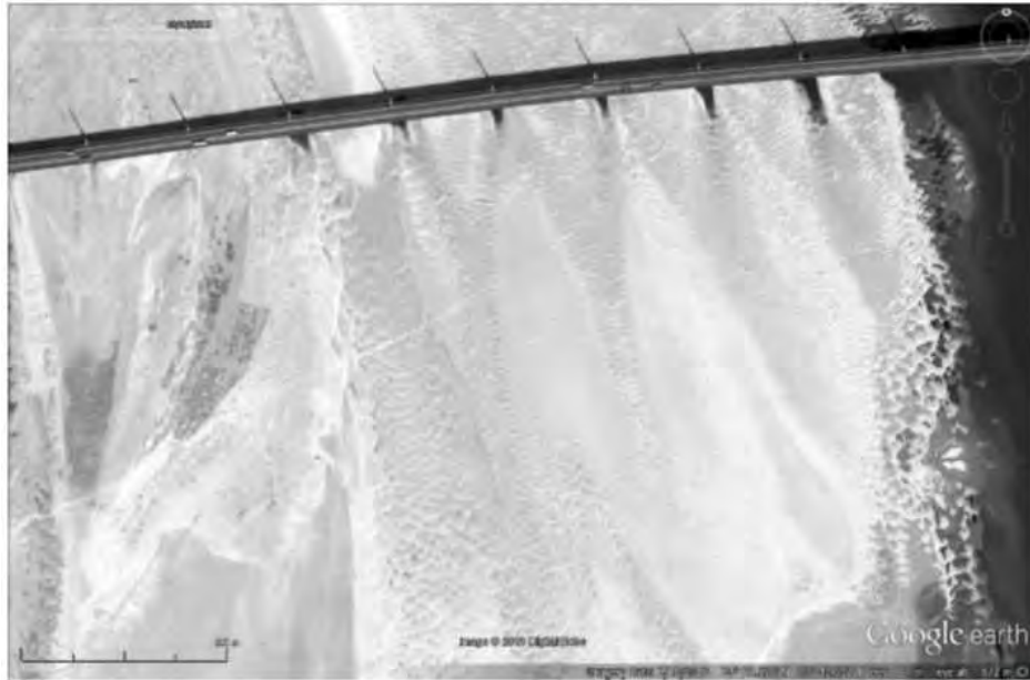
Figure 13.13: Scour and Deposition Patterns on Sand Bar Downstream of the Existing Bangabandhu Bridge. (Pier Spacing = 100 m, Scale Length = 200 m). Flow from Top to Bottom of Image
