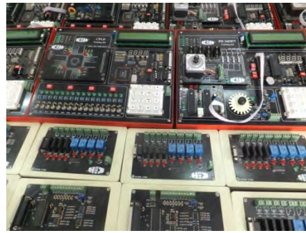
Photo 2-3: PLD (upper left) and PIC (upper right)
