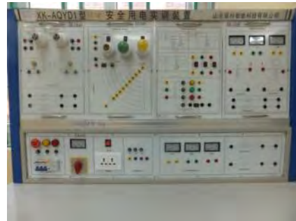
Photo 13-1: Electrical safety training device and program
