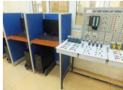
Photo 13-2: PLC motor speed controller development computers
