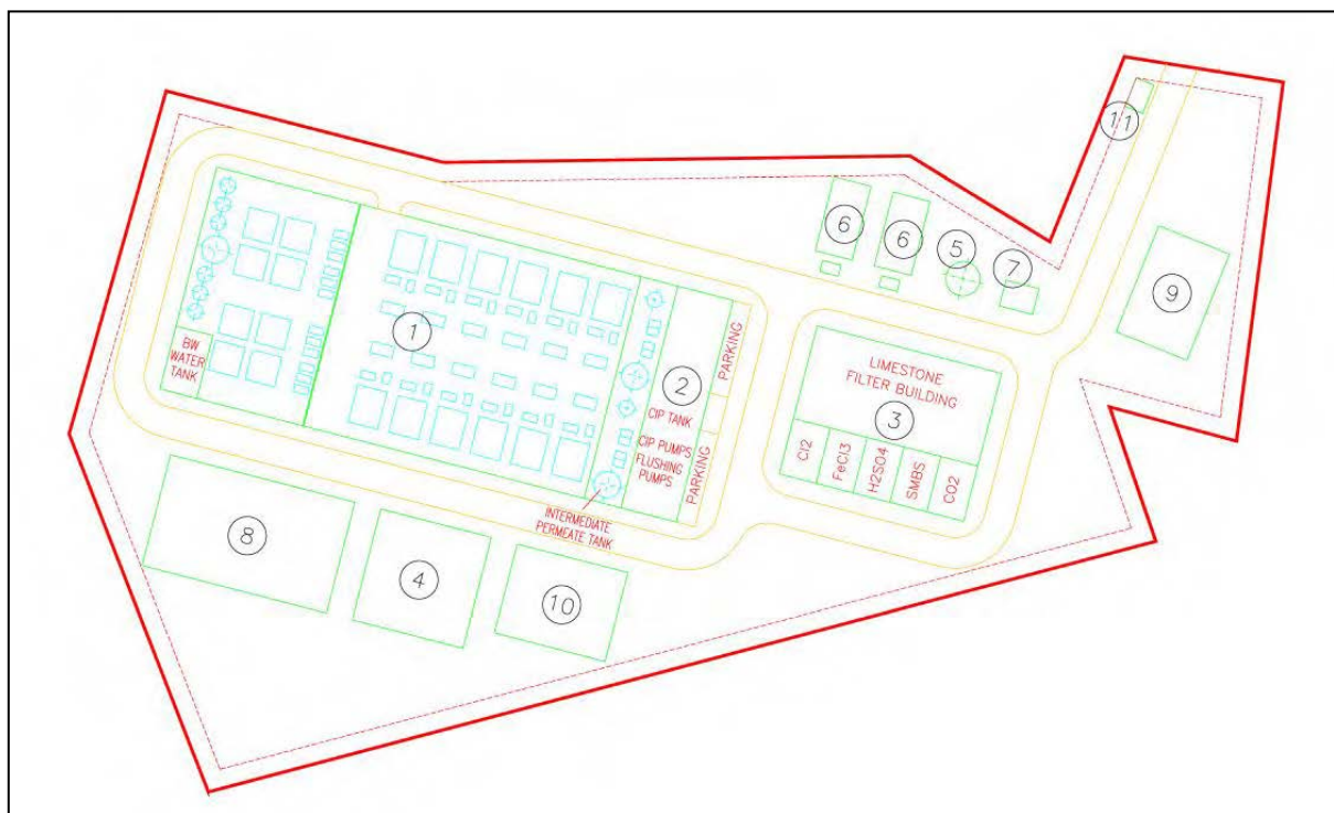
Figure 5.1.3 Layout Plan of the Mamelles SWRO Plant
