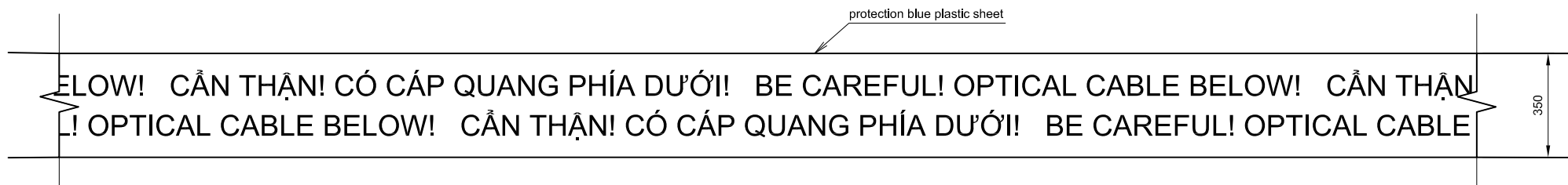
PROTECTION BLUE PLASTIC SHEET scale:1/20
