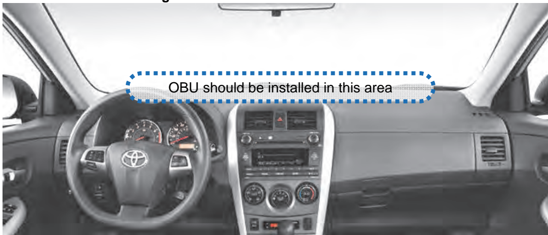
Figure 7.3 Installation of OBU in Vehicle
