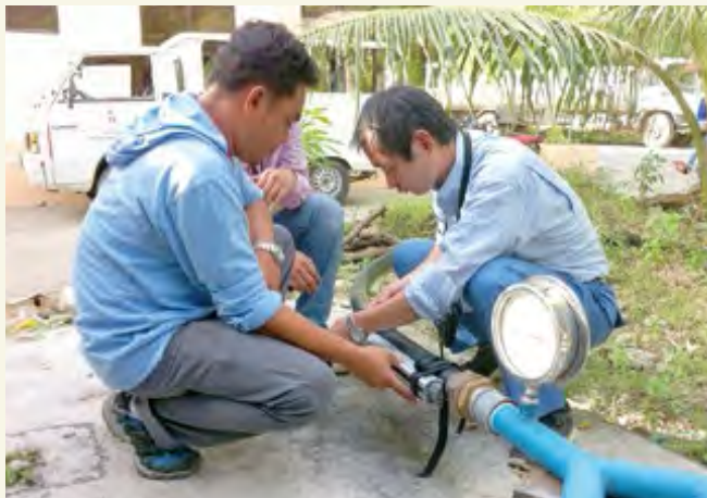
A mission member of Yokohama Water measuring flow velocity using an ultrasonic flowmeter in Cebu
