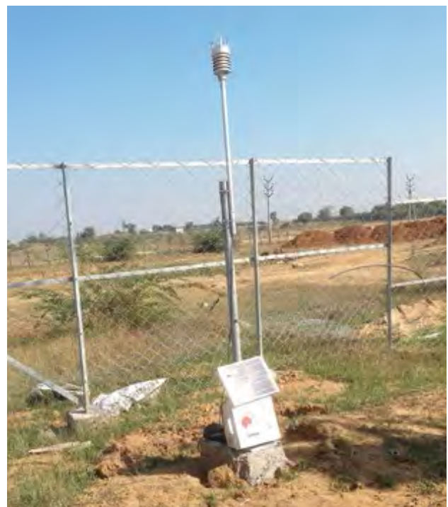
An Automatic Weather Station (AWS) set up under the research project Information Network for Natural Disaster Mitigation and Recovery in India.
