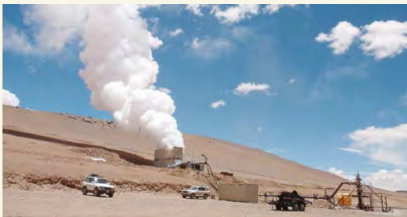
Conducting a well testing
