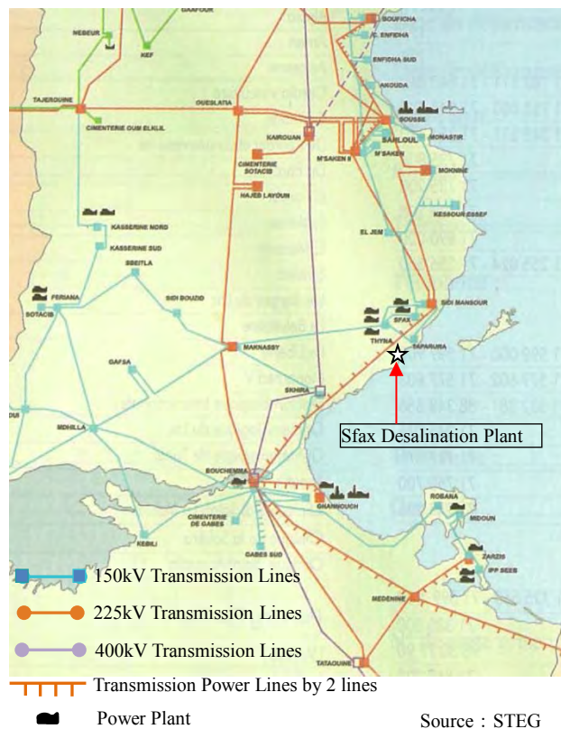
Figure 7.2-1 STEG Transmission Lines
