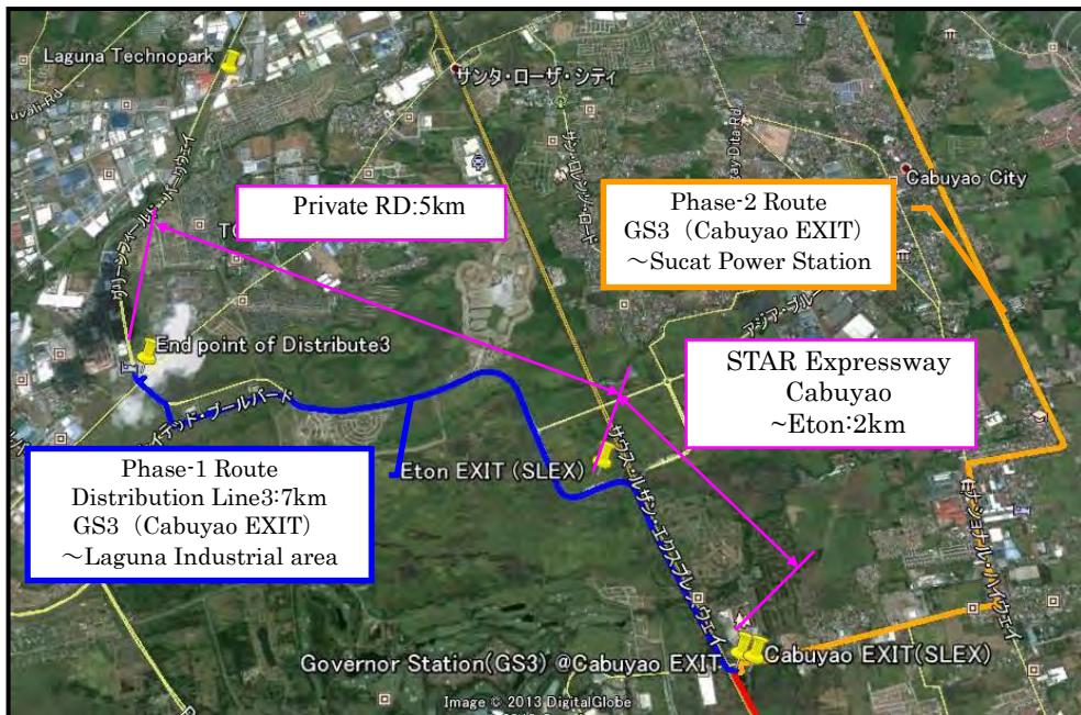
Figure 2.4-31 Route Survey Results (Distribution 3)
