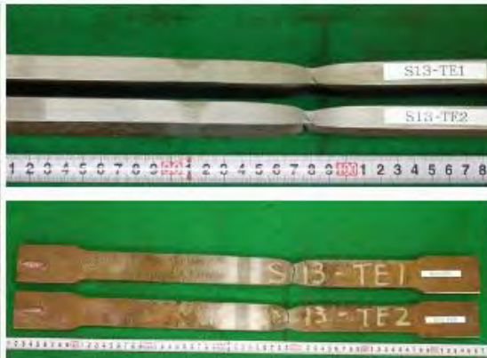
Test piece for tensile test
