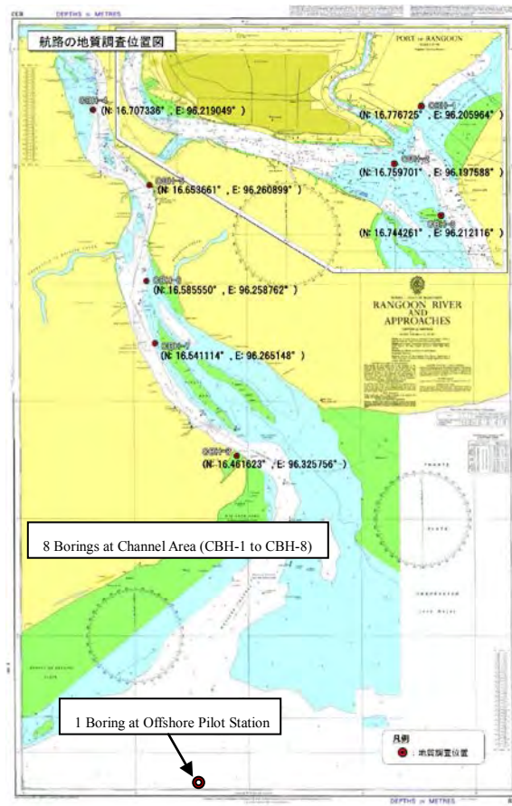
Figure 7.2-3 Location Map of Channel Area and Offshore Pilot Station
