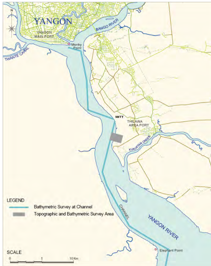
Figure 7.3-2 Location Map of Topographic and Bathymetric Survey
